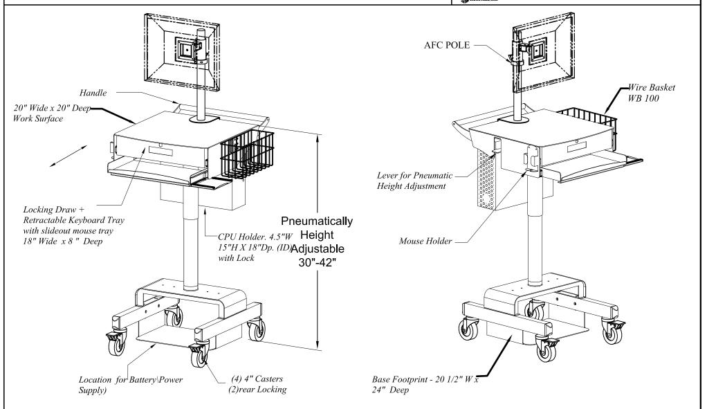
MATERIAL: DRAWN BY: MK DATE: 12/16/09 DESCRIPTION: NOTES: AS NOTED ABOVE Point of Care Cart V E D 0 USED ON : TOLERANCES UNLESS OTHERWISE SPECIFIED ENG: MFG: FRACTIONAL 2 PLC. DEC. 3PLC. DEC. Maxflex\PC500\wDR&KB ±.001 QA: PDF NAME: PC500-F-KB-DRW-CPU-WB-01 REV: SIZE SCALE : N.T.S. SHEET: 1 OF 1 **FINISH**
