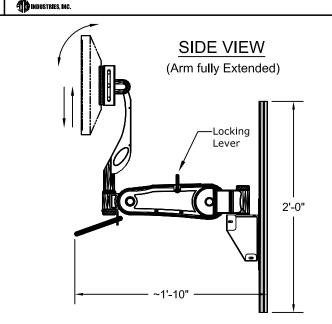
Pneumatically height adjustable arm with lock for varying loads-
