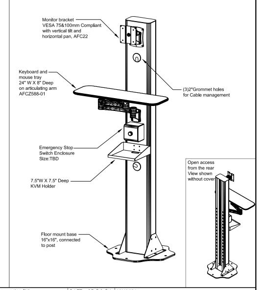
MATERIAL: NOTES: DRAWN BY: VGM/PR DATE: 05/19/11 AS NOTED ABOVE FLOOR POST-200 series A P Ρ R O V E D TOLERANCES UNLESS OTHERWISE SPECIFIED USED ON : ENG: MFG: 2 PLC. DEC. CUSTOMERS\HP SCITEX ±.50 QA: REV: 2 PDF NAME:
